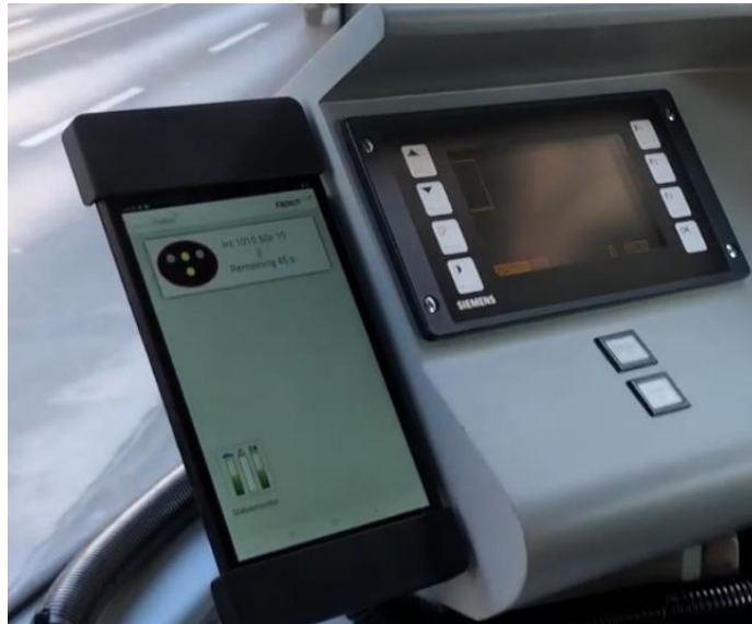
Figure 7: On Board Unit with tramway signaling
