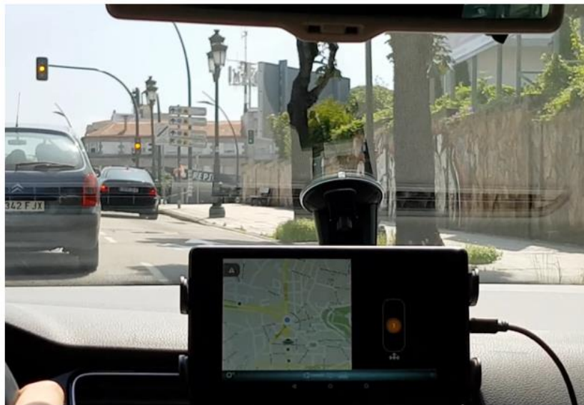
Figure 36: Operation of Time To Green in the SISCOGA Extended pilot.
